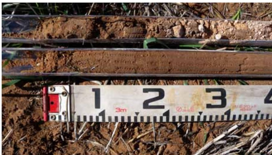
Figure 2: 0-40 cm soil cores extracted during sampling. Photo: DPI.
