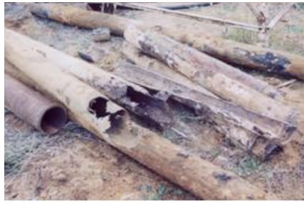
Above: Bore casings removed by the jacking procedure. The deterioration of the bore casings is clearly visible.
