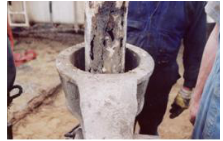
Above: Bore casings removed by the jacking procedure. The deterioration of the bore casings is clearly visible.
