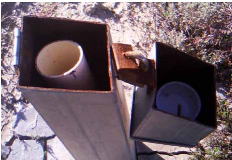
Above: A bore that has been opened for monitoring. Photo: Mallee CMA.
